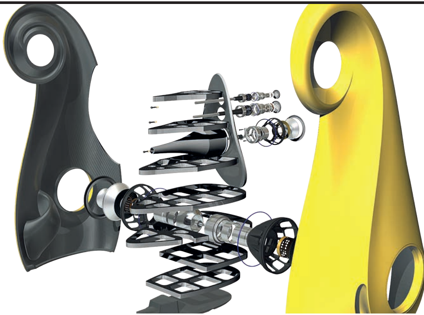
ABOVE: The Spirit's cabinet is fashioned from a rigid but lightweight sandwich of balsa between layers of GRP. It is internally reinforced by a series of carbon-skinned composite grids
